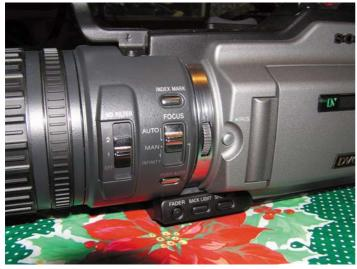
Additionally the black and white high-resolution viewfinder remains active when the LCD panel is open.
